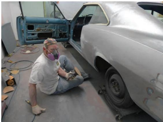
A typical workday here at Gopher Grove Garage would likely include rollin' 'round on a concrete floor while absorbin' all the not-so-good vibrations from pneumatic tools, like a DA (dual-action) sander, or worse. A particulate respirator is a must for survival, but it'll raise the body's operatin' temperature as recirculated hot breath has its side-effects.
