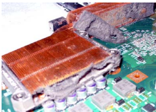
Laptop Cooling fins covered in dust
