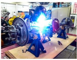
For this story's first installment, we'll conclude right here with coilover shock brackets, hairpin brackets, and the modified Panhard rod bracket welded in place.
